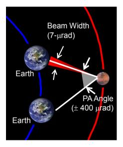
**Figure 4: Point Ahead Angle Example**
