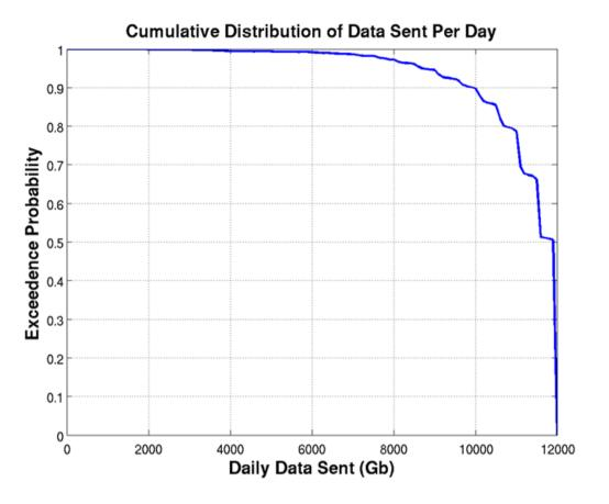
Figure 24: The cumulative distribution of the amount of data successfully sent to the ground by the LEO satellite for the nine-site network of ground stations.
