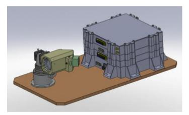
Figure 19: Schematic diagram of the terminal consisting of the optical head on a 2-axis gimbal (left) and an electronics/laser box (right).
