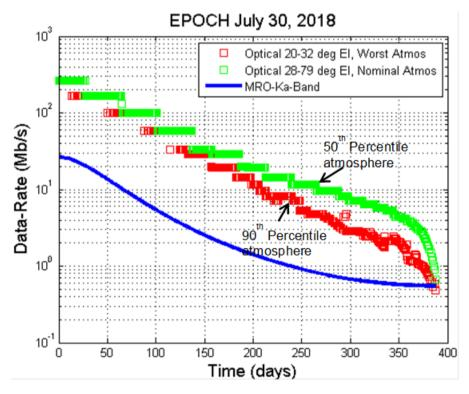
Figure 42: Data rate vs. distance at GDSCC
