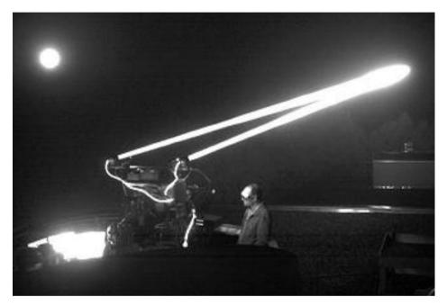
Figure 21: DLR's OGS at Oberpfaffenhofen during a laser link with the OICETS satellite at nighttime (2009). The two infrared uplink beacons can be seen.
