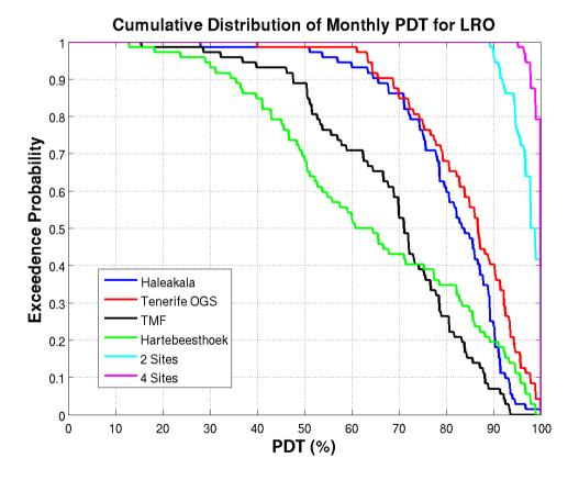
Figure 31: CDF of PDT for the four individual sites and the two- and four-site networks for the Lunar (LRO) scenario.
